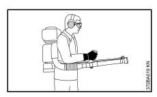
Carry the power tool on your back with both harness straps – do not hang it over one shoulder. Hold and control the blower tube with your right hand on the control handle – even if you are lefthanded Walk slowly forwards as you work – observe the nozzle outlet at all times – do not walk backwards – **risk of stumbling**.
