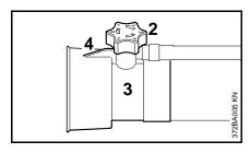
The discharge rate can be infinitely varied by turning the metering knob (2) on the nozzle (3).
