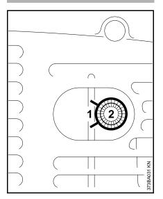
If the engine is down on power or does not run smoothly at maximum RPM, check the spark arresting screen (not fitted in all versions) in the muffler.
