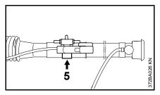
Tighten down the clamp screw (5) (see "Adjusting the Control Handle").
