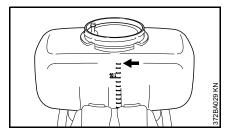
Fill up with thoroughly mixed spray solution – do not exceed 13 liter mark (arrow).
