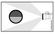
Splits the spray jet in two – allows two closely planted rows to be treated in one pass.
