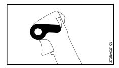
Move the setting lever to the idel position.
